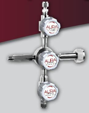
The AURA Deep Purge incorporates a unique snorkel tube design which forces the purge gas all the way back through the inlet connection to the cylinder valve cavity assuring virtual zero dead space purging. The Deep Purge may be used to purge the entire regulator body or just the cylinder connection at the time of cylinder change. The Deep Purge performs a positive displacement purge of the system.
